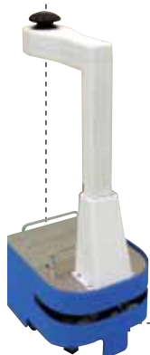
A lead-robot with obstacle avoidance capabilities
